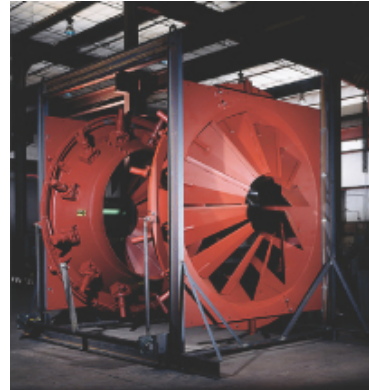
Efoxx Rotary Vane Damper for a Power Generating Plant
